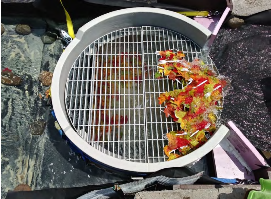
Figure 38. Rain Guardian Turret testing at 0.25cfs (RGT-025-A).
