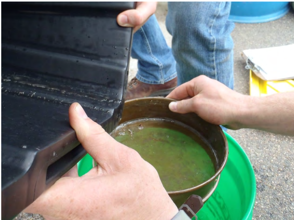
Figure 26. The rinse bin was poured carefully through a #325 sieve to retain sediment particles.
