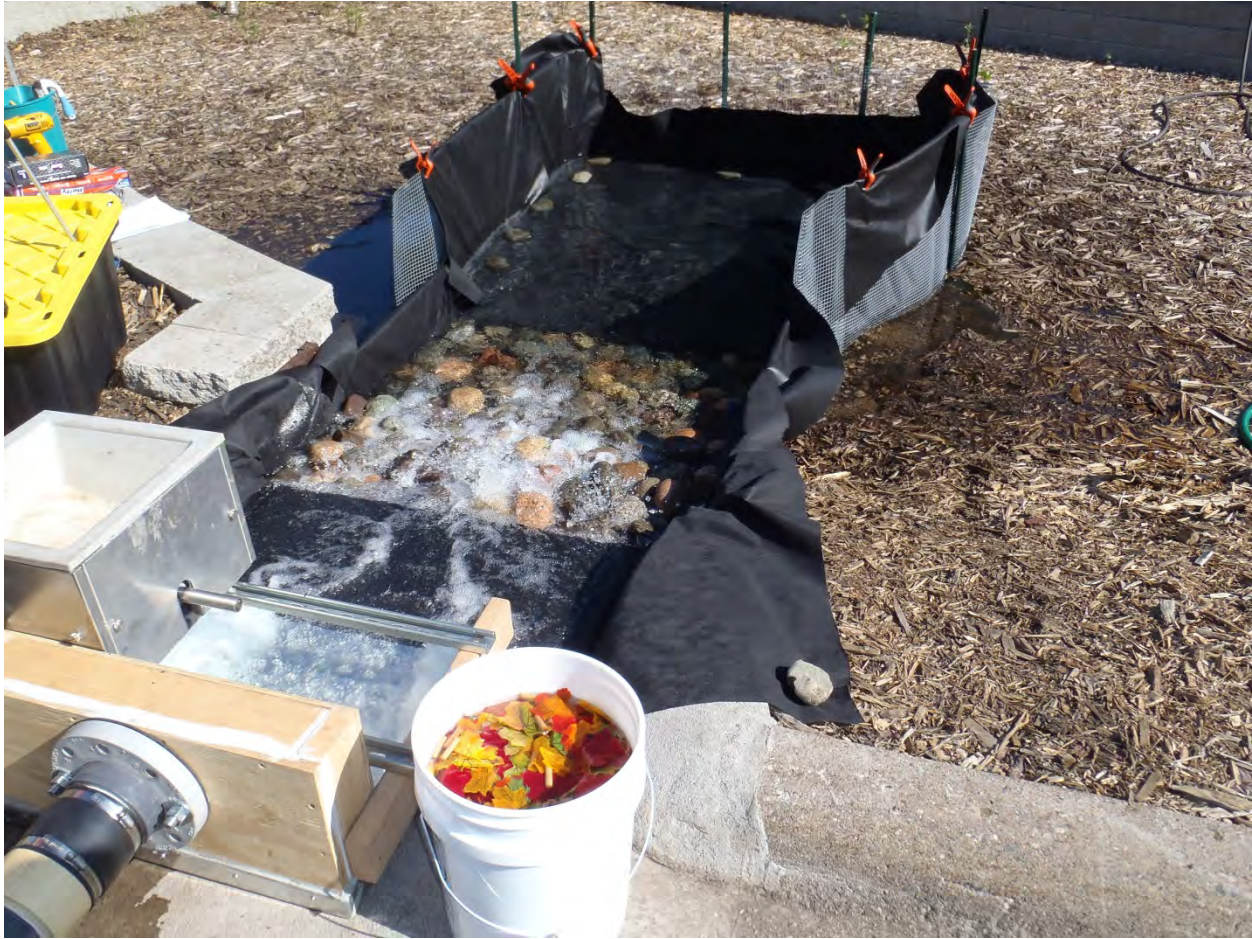
Figure 41. Beginning of flow on RLI, just prior to the start of a test. Gross solids and sediment are ready to be fed.
