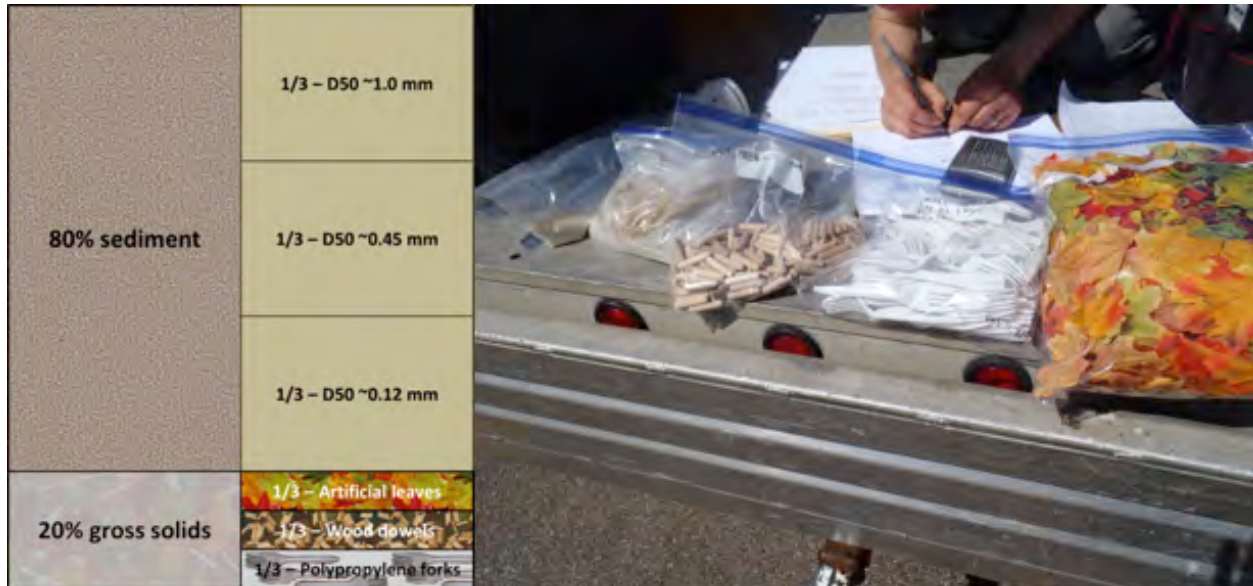
Figure 15. Synthetic stormwater solids composition. The height of each labeled box (left) is mass-proportional to the amount used in testing. The picture at right shows approximately the volume used of each component.
