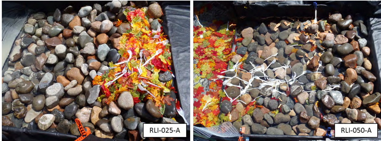
Figure 42. Rock lined inlet after testing at 0.25 cfs for 40 minutes (left) and 0.50 cfs for 20 minutes (right).
