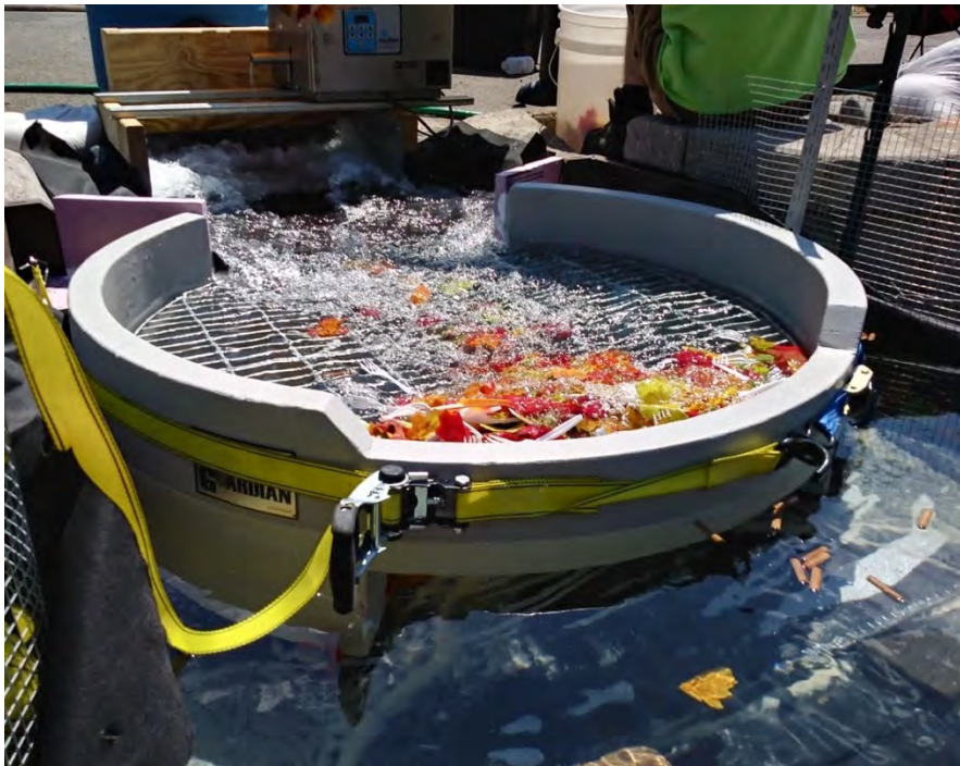
Figure 39. Rain Guardian Turret testing at 0.50cfs at a high water level (RGT-050-B).
