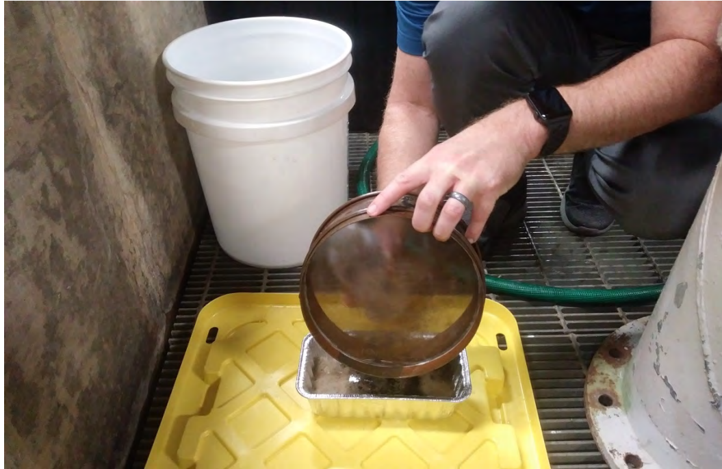
Figure 28. Rinsing sediment from a sieve into a pan for oven drying.
