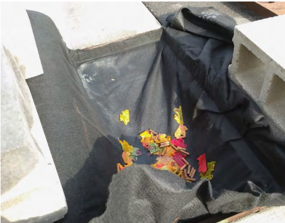
Figure 50. Gross solids and slight amount of sediment captured on geotextile fabric in the downstream catch basin frame (BBP-012-A).
