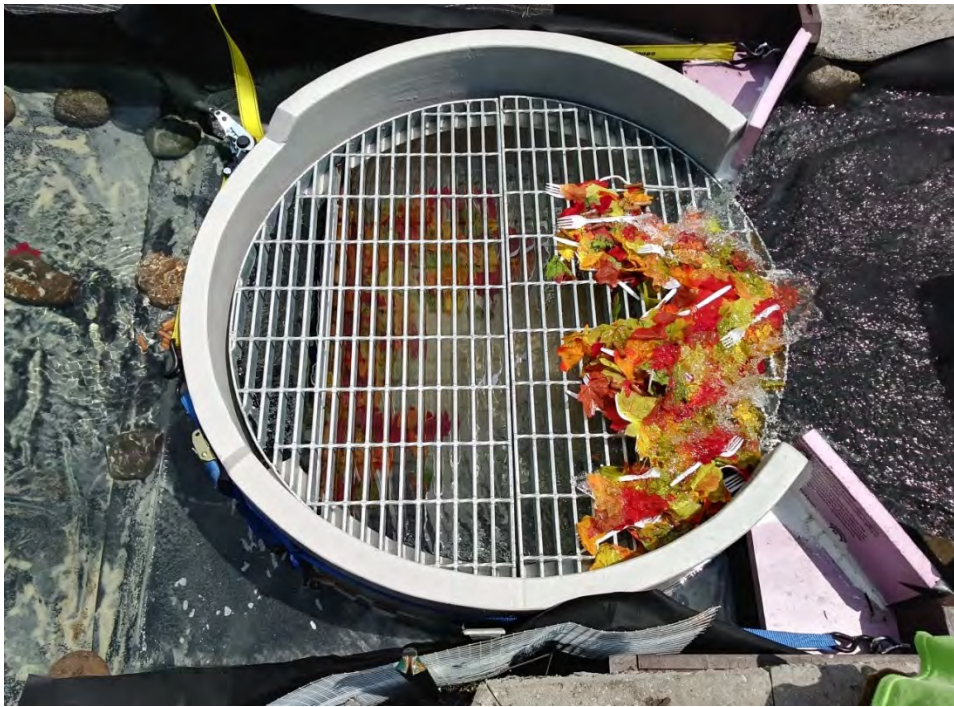
Figure 10. Rain Guardian Turret testing at 0.25 cfs (RGT-025-A). Entrance from the curb cut comes into the RGT from the right of the picture; flow through the screen wall exiting the RGT in the center of the picture towards the left.
