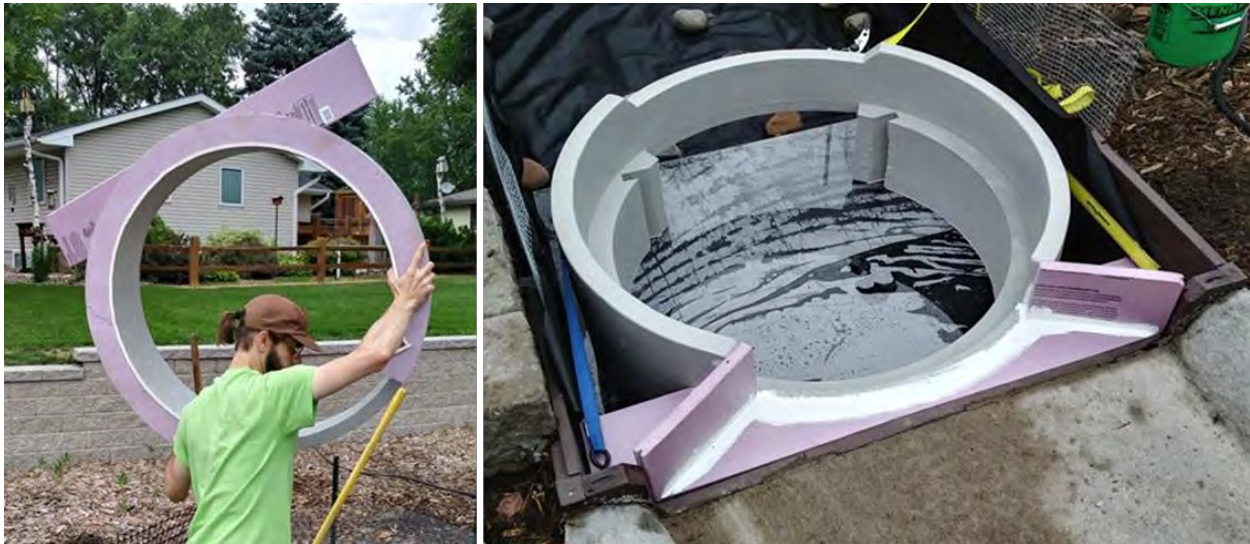
Figure 37. A special lightweight replica of the Rain Guardian Turret was used in testing at the Anoka site.
