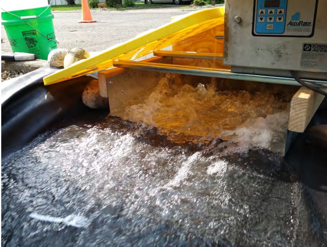
Figure 22. Sediment feeder and flow distributor.
