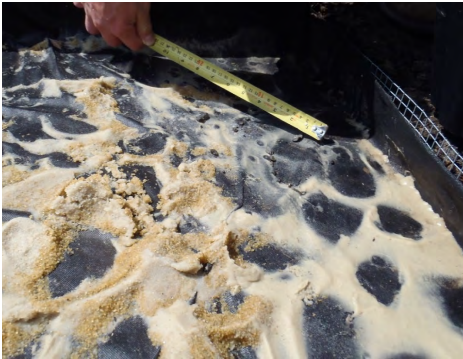
Figure 45. Sediment remaining on geotextile when rocks were removed from RLI.
