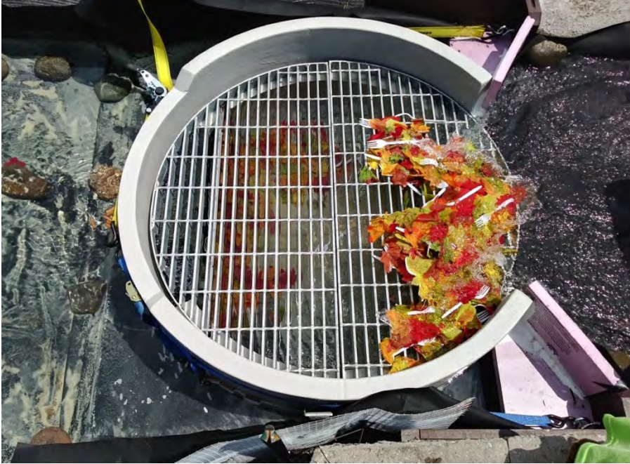
Figure 38. Rain Guardian Turret testing at 0.25cfs (RGT-025-A).
