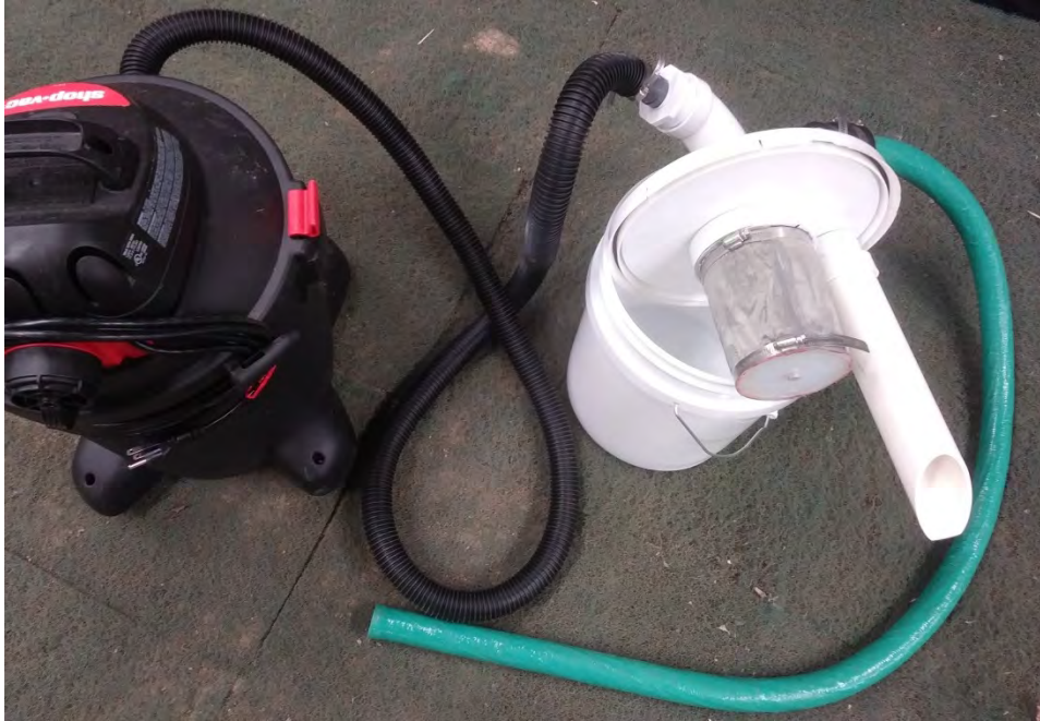
Figure 24. A filter bucket was designed to trap sediment in the 5-gallon bucket (right), with suction provided by a wet-dry vac (left).
