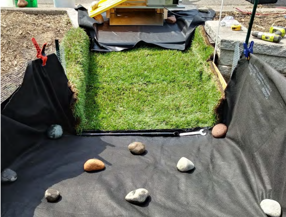
Figure 32. Grass lined inlet with fabric lined corral, after rinsing, ready for a test.
