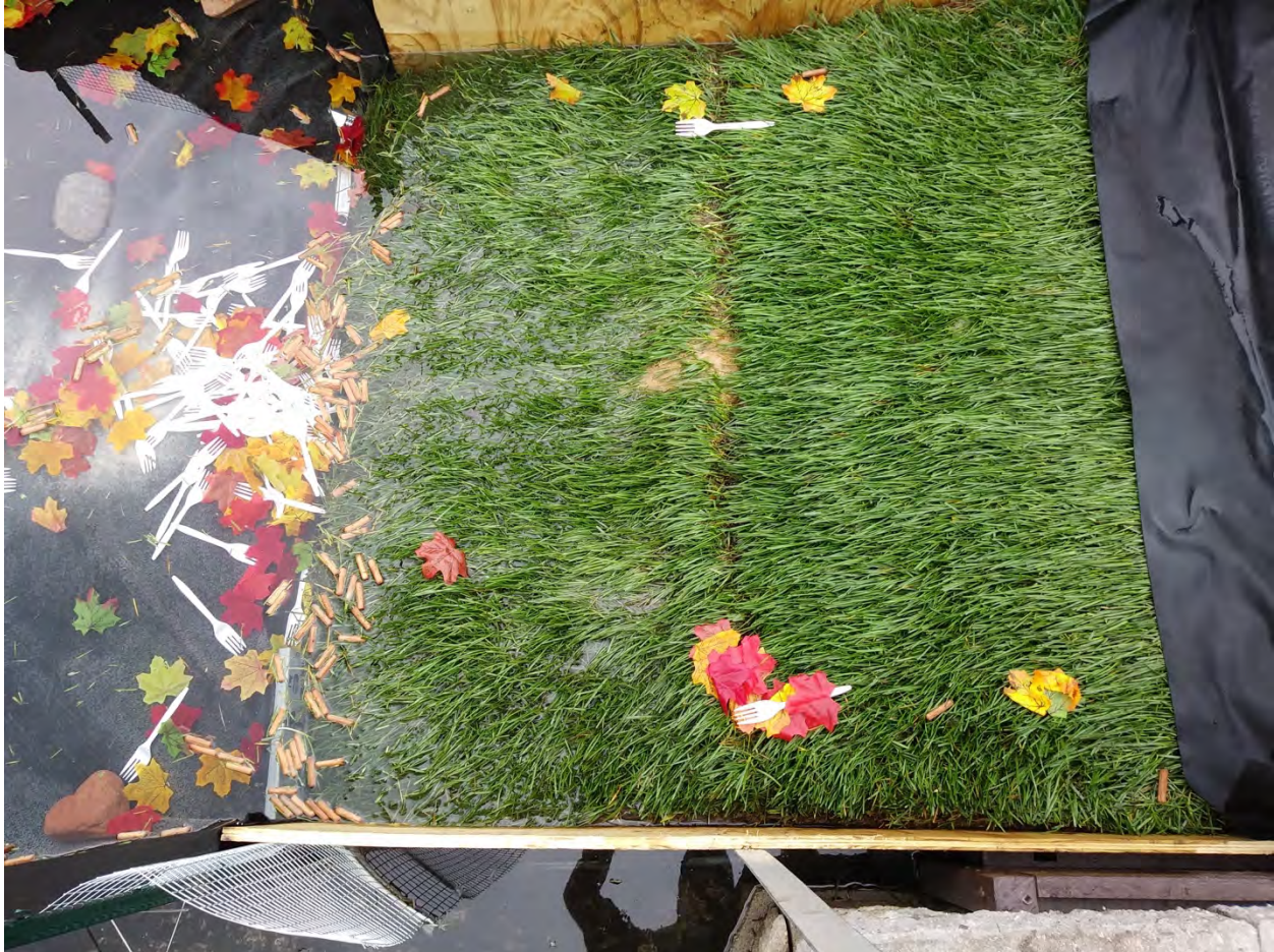
Figure 55: Capture of gross solids on grass lined inlet. Note wood dowels floating on water surface above the GLI near the downstream boundary with the corral. These dowels were deposited on the GLI during drawdown and counted as "captured."
