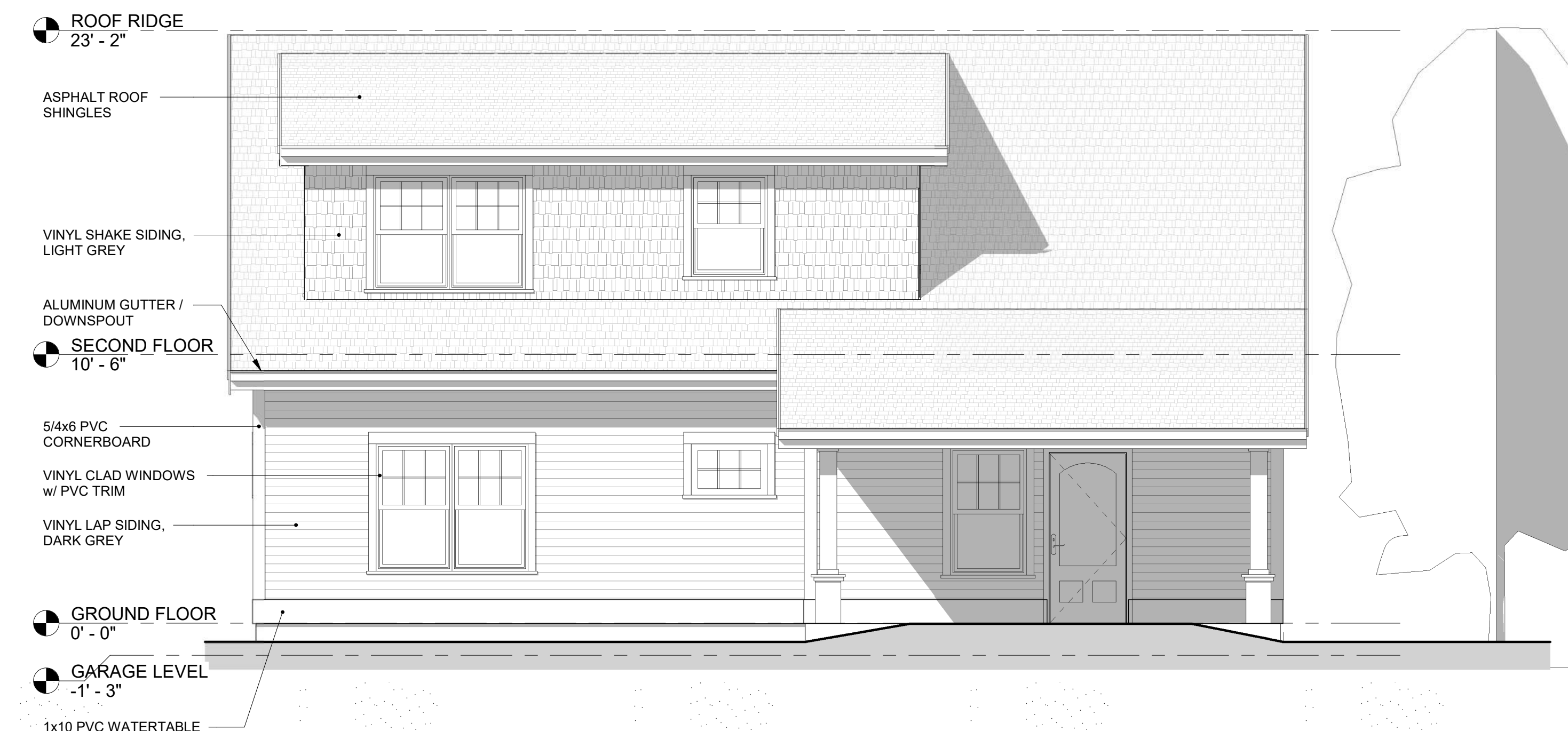
3 ELEVATION FACING GREEN SPACE 1/4" = 1'-0"
