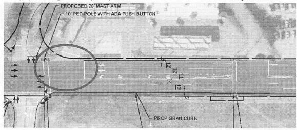
Appendix B SFEIR proposed design that removes the safety elements of a separate traffic phase and traffic break for vehicles exiting Interstate and traveling Northbound.
